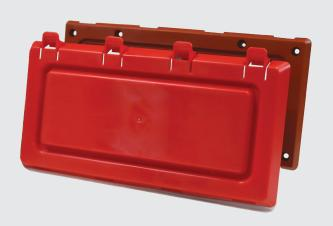
The Fernco Anti-Flood Air Brick Cover comes in two parts, a terracotta coloured frame which permanently fixes around the existing air brick and a red coloured cover which is designed to be clipped onto and seal against the frame during a flood event. After floodwater subsides, the cover can simply be unclipped and stored ready for future flooding events.
