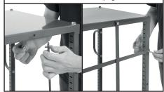
Start to position the tray runners where required in the slots on the uprights. Ensure they are level on each upright to avoid slanting boxes
