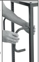
Attach the rear retaining bars into the holes provided, on the opposite side of the handles, using the appropriate fixings: short bar requires M6 bolts, nuts and a 10mm spanner, the larger bar requires 45mm M8, nuts and a 13mm spanner. Ensure the shorter retaining bar is fixed in the lower two holes on the uprights
