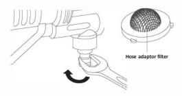
3-2. Clean hose filter regularly to avoid blocking hose inlet. Rotate hose filter cover to detach from hose, take out the hose filter and clean it.
