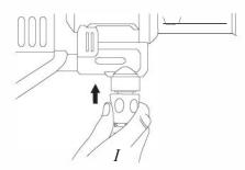
3-2.Disconnect hose: Hold hose connector, pull it away from hose adaptor.
