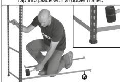
Beam Ties (1525mm wide shelving only). Attach one end of the beam tie to the slot in the centre of a single front beam and tap into place in the end frames. Then fit the other end of the beam tie to the centre of the rear beam before tapping into place in the end frame (as shown).
