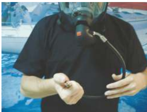
Figure 13 Face piece leak tightness test
