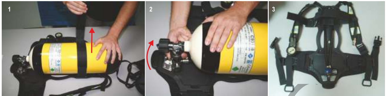
Figure 24 Removal of empty cylinder from apparatus
