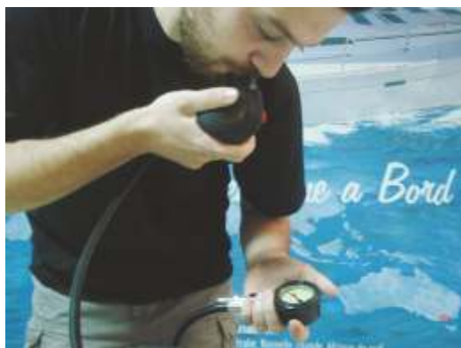
Figure 9 "ON DEMAND" valve operability check
