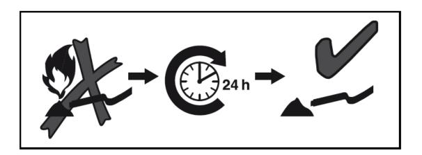
Wait at least 24 hours before vacuuming an oven or a fireplace in order to be sure that the fire has gone out and the ash has cooled down. Only for cold ash, refer to the following operating instructions!
