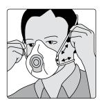
4. Adjust strap by pulling loop on strap.
