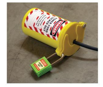
This large Electrical Plug Lockout has 2 interlocking cover plates allowing plugs with various sizes of cable to be inserted. Interior size of 84mm dia. x 150mm and will accept cable widths up to 34mm dia.
