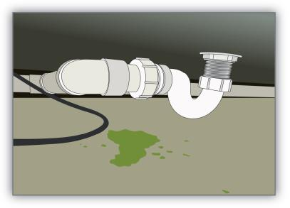
The green dye will quickly identify leaks, the dye is UV sensitive and can be used in conjunction with UV light to locate the smallest of leaks.
