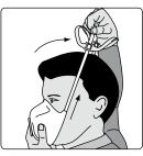
Place respirator on chin and pull head strap on the head harness over the crown of the head.
