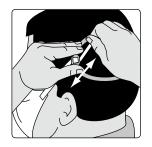
Ensure the respirator fits securely and comfortably. If necessary, adjust strap by pulling it at either side of the head harness.
