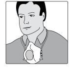
Unbuckle to take off. During work breaks open the buckles and let the mask hang around the neck.
