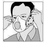
4. Ensure respirator fits secure and comfortable. To fasten respirator pull strap at either side of the buckle.
