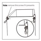
7. Unscrew and remove the bottom hinge pin, turn the bracket over and replace i
