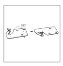
4. Unscrew middle hinge. Then lift lower door and place it on a soft pad to avoid scratching.
