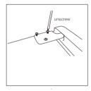
3. Remove the pin with a screwdriver and flip t hinge bracket. Then refit the pin to hinge bracket.
