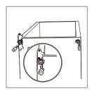
9. Make the middle hinge reverse the direction 180 oC then transfer it to the left property position. Place the middle hinge pin in the upper hole of the lower door, then tighten the bolts.
