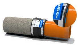
**4.** Position the smaller pipe, ensuring the coupling face and marked line are flush. Tighten this clamp band.
