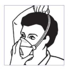
3. Cup respirator under chin. Ensure the two straps are separated and pull the straps over the head, one at a time.
