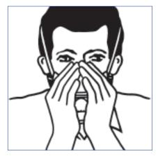
6. To check fit, cup both hands over the respirator and inhale sharply. If air flows around the nose, re-mould the nosepiece.
