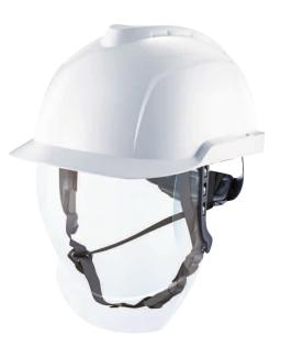
Balanced lightweight electrician's safety helmet, non-vented, with 6-point Fas-Trac® III ratchet suspension and GS-ET-29 class 1 face shield certified for protection against arc flash. For use where top impact hazards to the head, chemical splash, Ultra-Violet radiation, molten metal splash or electric arc to the face exist.
